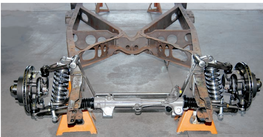
27) The chassis is finished and the HEIDTS® suspension looks great and works terrific. The '40 will have positive power steering, should handle like a sports car and will stop quickly with the large brakes. The best part is this kit is priced right.
