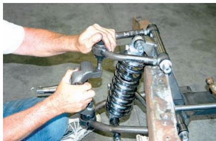
19) Now the upper A-arm can be connected to the spindle. HEIDTS® recommended using one of its narrow front suspension kits to keep the tires inside the fenderwell so the tires don't hit on turns.
