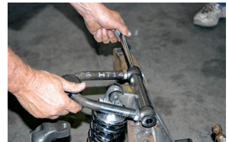
18) Using the other long bolt supplied in the kit, the upper A-arm was installed. This connection also uses the large washers supplied in the kit. The upper bolt is secured with a Nvlok locknut.
