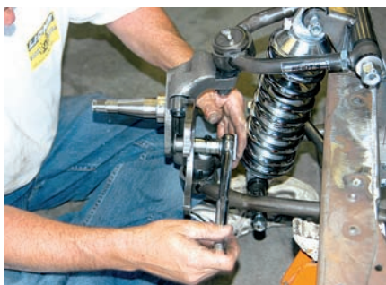
20) The caliper bracket is designed with one bolt on the top traveling upward into the spindle and another bolt on the bottom with a bolt that travels sideways into the spindle.
